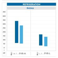
Testing conditions data reference: M.T. : evap. T. -10°C; cond. T. +45°C L.T. : evap. T. -35°C; cond. T. +40°C ECO
