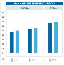
Testing conditions data reference: M.T.: evap. T. -10°C L.T.: evap T. -35°C
